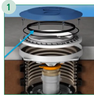
Remove Upper Bolts and Ring
